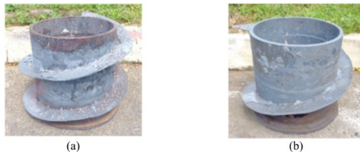
FIGURE 4. Spiral finned crucible pot: (a) inclination angle 10^\circ , (b) inclination angle 15^\circ
